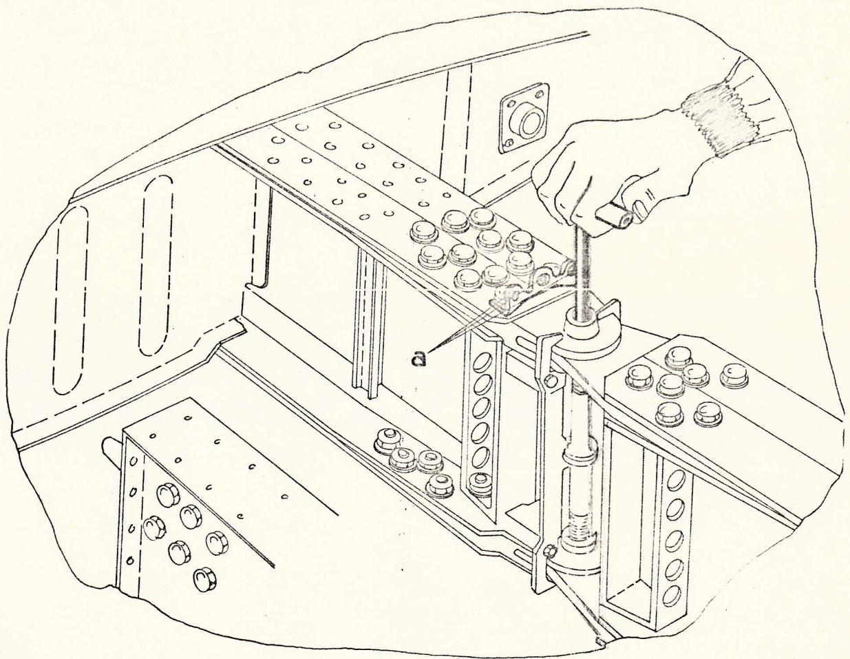
Fig. 6.2.1 Main junction tightening
